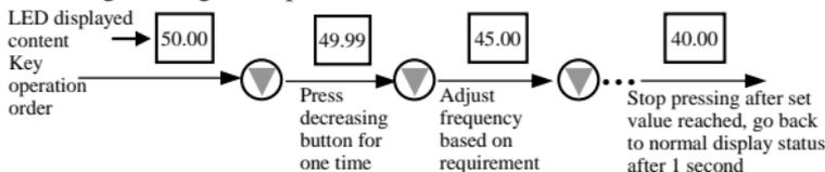
**Fig. 4-8 set frequency adjustment operation example**
