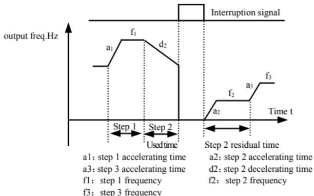
**Fig.6-25 PLC starting mode 1**
