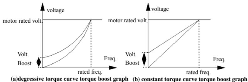
**Fig.6-4 torque boost graph**
