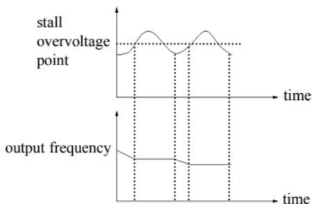
**Fig.6-40 overvoltage stall function**
