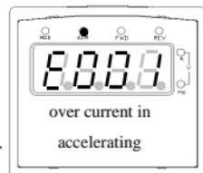
Fig.4-4 failure alarm
