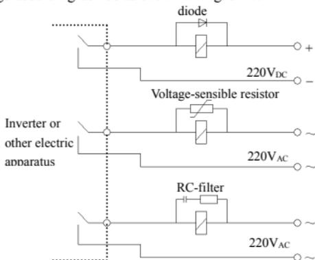
Fig.3-17 installation demand for electromagnetic on-off device
