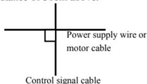
**Fig.3-16 system wiring demand**
