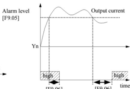
**Fig.6-38 electronic thermal relay protection** **Fig.6-39 overload alarm**
