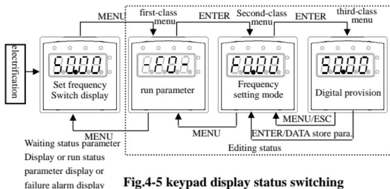
Fig.4-5 keypad display status switching
