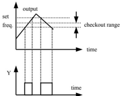
Fig.6-34 freq. arriving signal output
