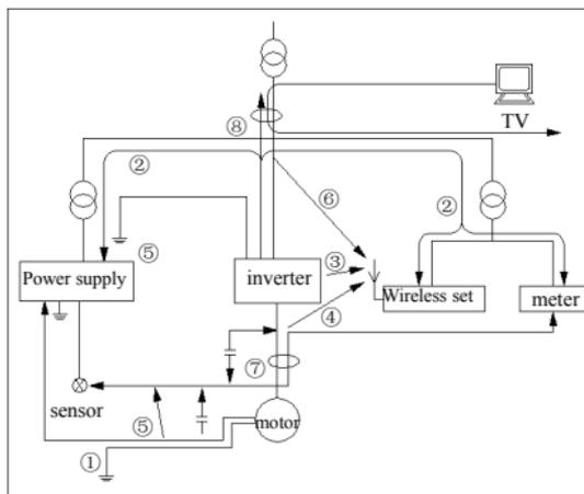
Fig.3-15 noise disturbance spread road sketch
