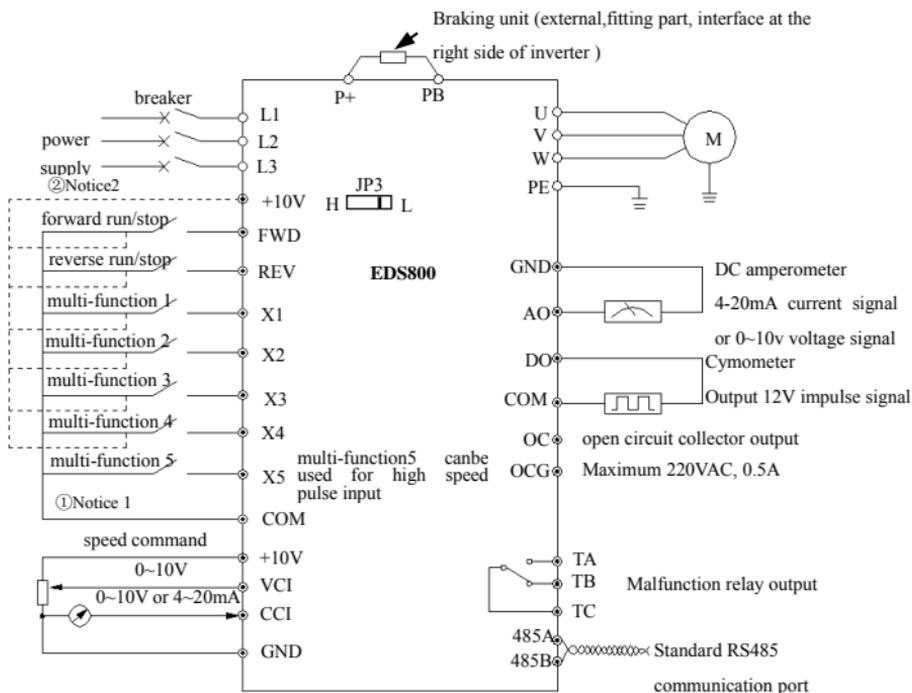
**Fig. 3-6 basic wiring diagram**
