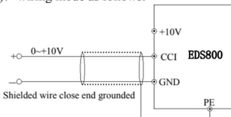
**Fig.3-9 CCI terminal wiring diagram**
