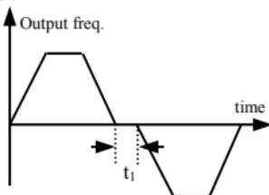
**Fig.6-9 FWD REV run dead-section time**
