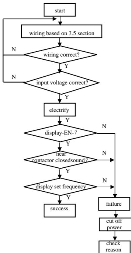
Fig. 4-12 first electrification operation flow
