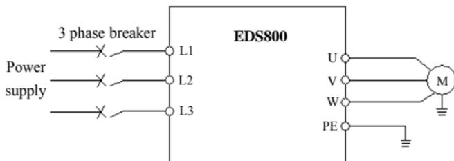
Fig.3-4 main loop simple wiring
