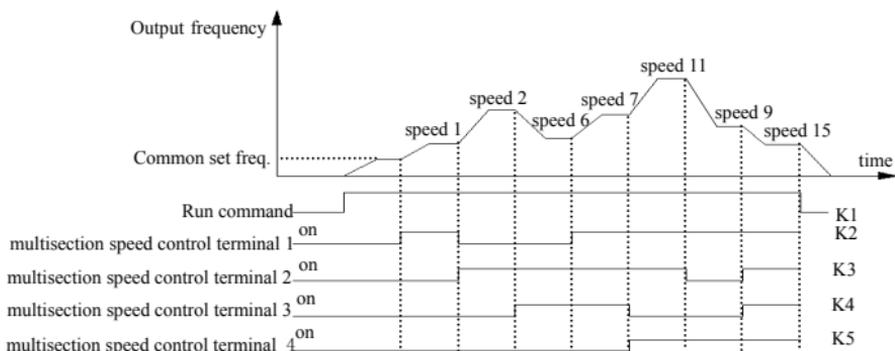
Fig.6-26 multi-step speed run
