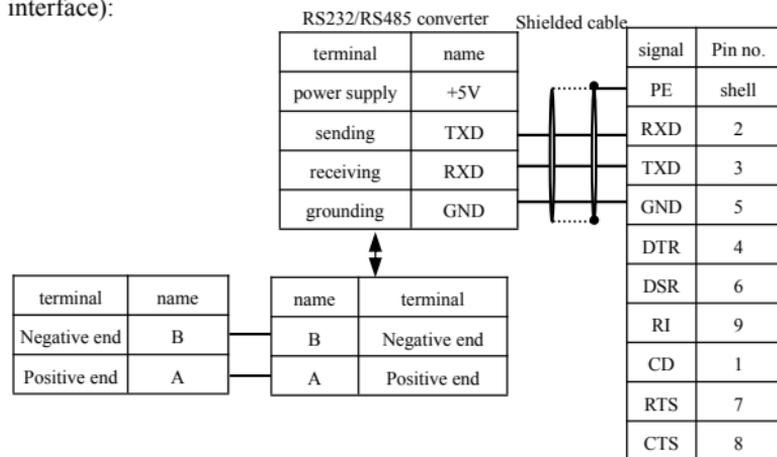
**Fig. 3-12 RS485 communication wiring**
