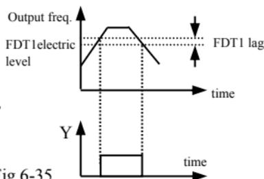
Fig.6-35 freq. level detecting
