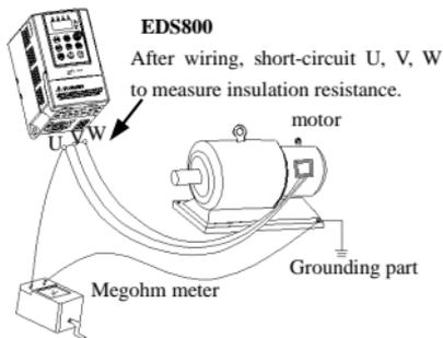
Fig.1-1 motor insulation measure
