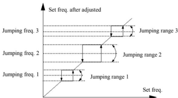
Fig.6-12 jumping frequency and range graph
