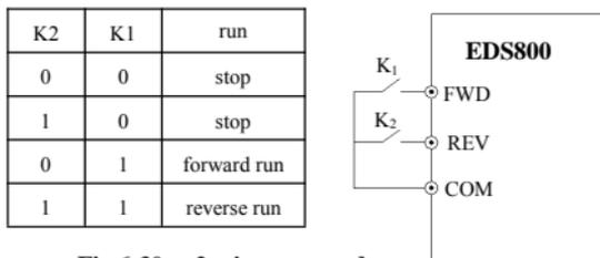
**Fig.6-30 2-wire run mode****2: 3-wire control mode 1**
