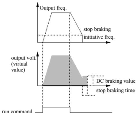
Fig.6-8 Dec stop+DC braking
