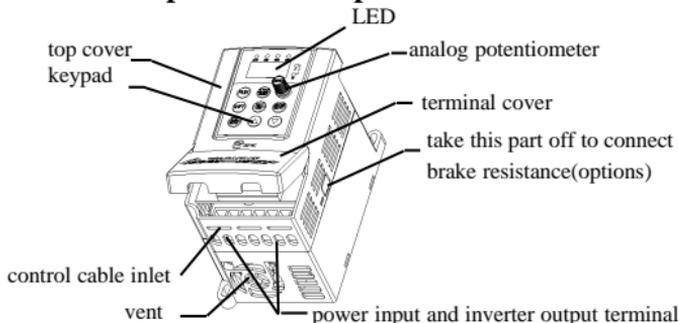
Fig. 2-3 Parts name sketch for EDS800
