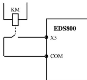
Fig.6-28 exterior device failure always-open input
