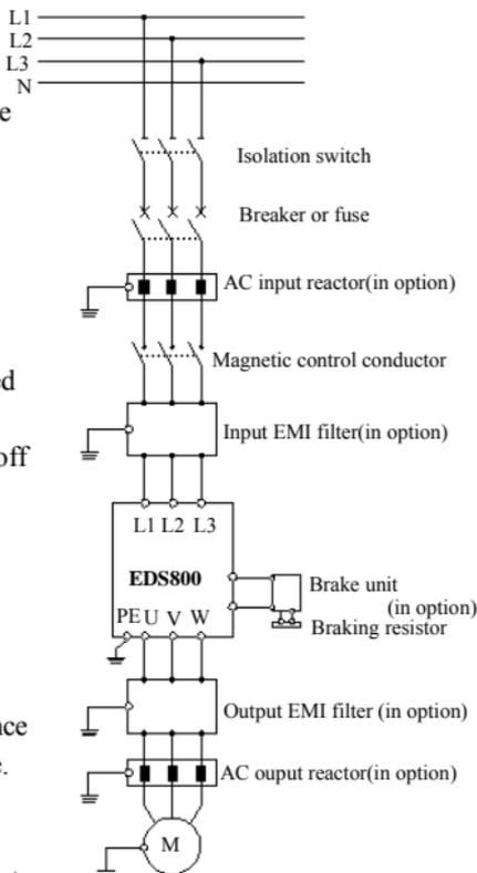
Fig.3-5 connection of inverter and fitting parts
