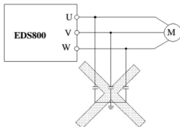
Fig.1-2 capacitor at output side forbidden
