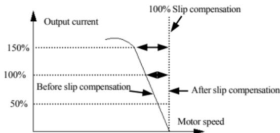
**Fig.6-10 slip freq. compensation graph**
