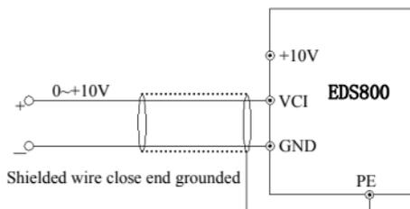
**Fig.3-8 VCI terminal wiring diagram**
