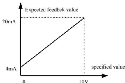
**Fig.6-15 specified value and expected feedback value**
