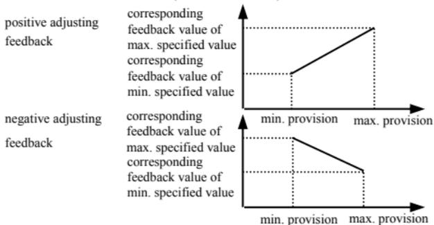
**Fig.6-16 provision, feedback curve**
