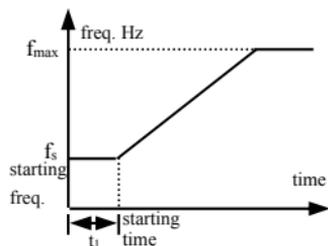
Fig.6-6 starting freq. and starting time
