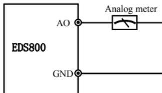
**Fig.3-10 analog output terminal wiring**
